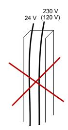
Not allowed unless the 24 V cable is insulated for 230 V (120 V) or insulated with an insulation sleeving for 230 V (120 V).
