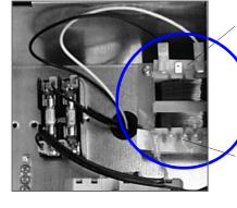
Set to 220 V if the supply frequency is 60 Hz. Set to 230 V if the supply frequency is 50 Hz.
