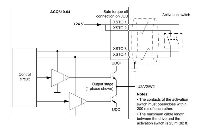
WARNING! The Safe torque off function does not disconnect the voltage of the main and auxiliary circuits from the drive. Therefore maintenance work on electrical parts of the drive or the motor can only be carried out after isolating the drive system from the main supply.
