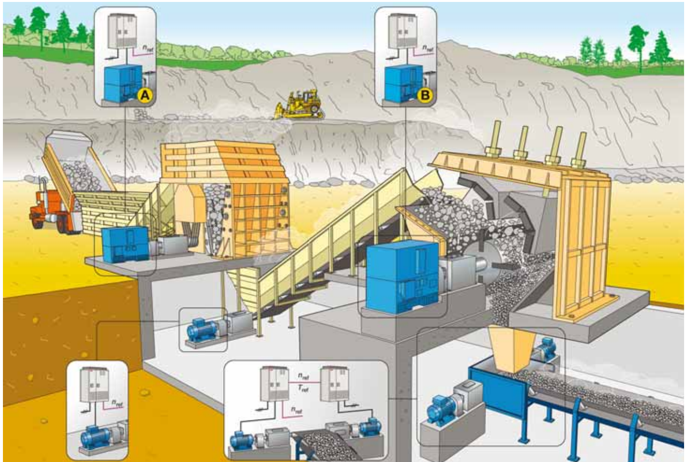
Motor control method A applied to a jaw crusher. Motor control method B applied to a hammer crusher.
