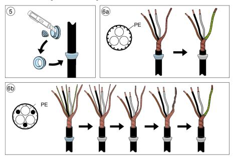
7. Slide the cable through the hole of the lead-through plate and attach the grommet to the hole.
