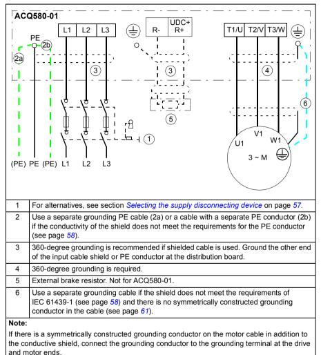
Do not use an asymmetrically constructed motor cable for motors above 30 kW (see page 58). Connecting its fourth conductor at the motor end increases bearing currents and causes extra wear.
