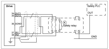
An example of a Safe torque off wiring with external +24 V DC power supply is shown below.
