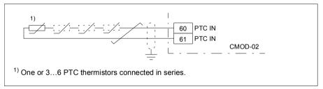
The PTC input is reinforced/double insulated. If the motor part of the PTC sensor and wiring are reinforced/double insulated, voltages on the PTC wiring are within SELV limits.
