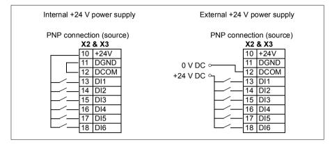
**WARNING!** Do not connect the +24 V AC cable to the control board ground when the control board is powered using an external 24 V AC supply.
